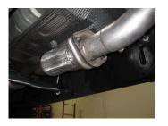
3. Install headpipe #A onto your existing stock 2-bolt flange. Use stock nuts to secure. Do not tighten
